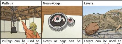
make a small force lift a heavier load. The more wheels in a pulley, the less force is needed to lift a weight.
